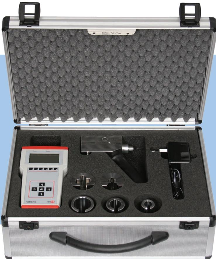
Three differently sized centring sleeves and two chain adapters for chain sizes of 3 x 9 ... 11 x 31 mm (in accordance with EN 818-2), a charger and 5 m signal cable make the chain hoist test set immediately and universally applicable.
