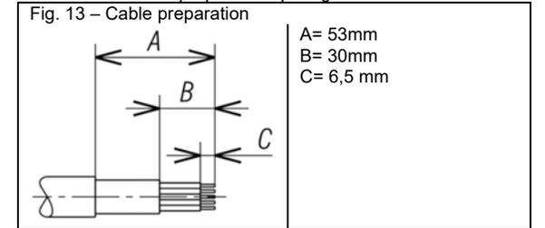
The single stripped conductor has to be crimped with each contact pin. For the electrical connections and for the assembly follow Fig.14.
