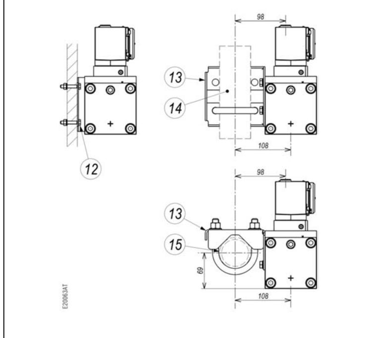
Fig. 10 – Switch equipped with capillary diaphragm seals
