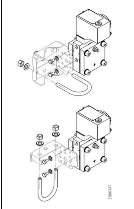
Fig. 9 – Typical Mounting
