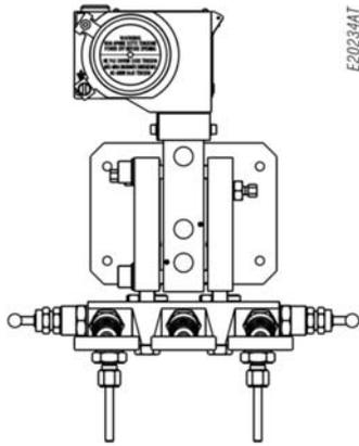
Fig. 13 – Assembly with swivel 1/2G manifold valve
