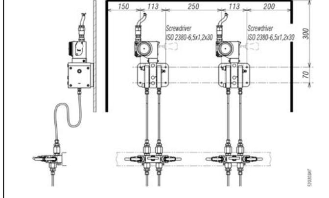
Fig. 12 – Assembly with flanged manifold valve
